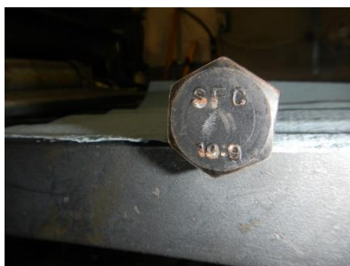
Metric bolt with a 10.9 grade marking, similar to grade 8 SAE bolt. The numbers are NOT the size, pitch, or diameter in metric, they only indicate the strength rating of the bolt.
