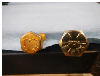
Six strike headed SAE grade 8 bolt. I use this grade of bolt for critical areas of assembly such as bolting the water tank in place. The lettering is from the manufacturer and has no bearing on strength, diameter, or thread size of the bolt.
