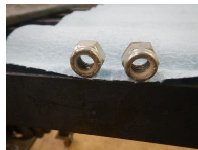
Nylock or Elastic stop nut, available in SAE and metric. These have a nylon insert that will hold the nut from vibrating loose. I use these in place of lock washers in high vibration areas such as the pump mounting bolts.
