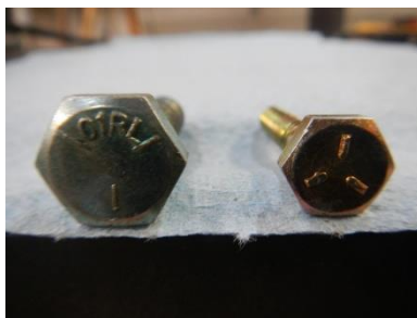
Three strike headed SAE grade 5 bolt. I use this grade of bolt for all general construction.
