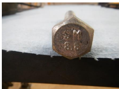
Metric bolt with 8.8 grade markings, similar to grade 5 SAE bolt. The numbers are NOT the size, pitch, or diameter in metric, they only indicate the strength rating of the bolt.
